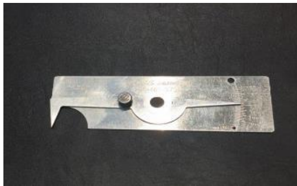
Figure 7.3-28 Welding Inspection Gauge
