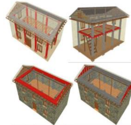
Primary elements of the standard type retrofit design: (Top row: althing beams, side strips; Bottom row: ring beams, lightweight gables)
